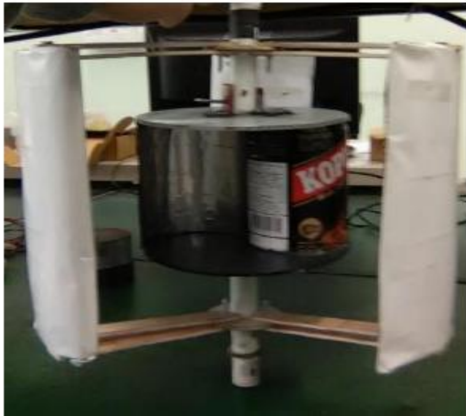
Figure 2.1: Hybrid Wind Turbine (Savonius -Darrieus) (Hidayanti et al. , 2020)
