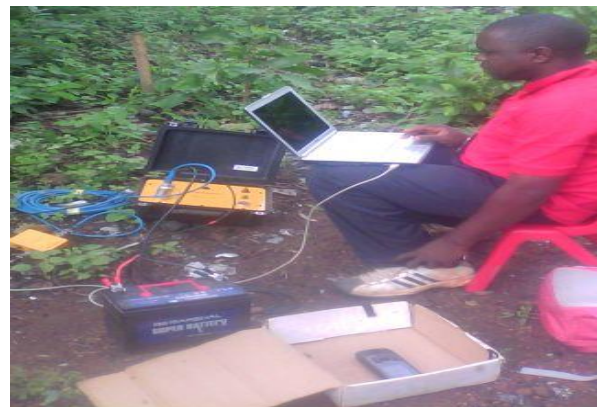
PLATE I: Seismic Refraction Tomography in Millennium City
