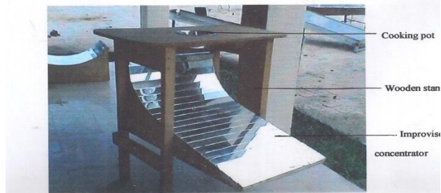
Plate 1: Constructed parabolic concentrated solar cooker
